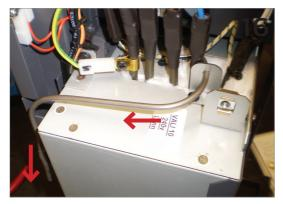
Now bend the pipe around the Heat Exchanger as shown.
