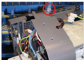
Gently manoeuver the Vertical Strap away from the left-hand side of the machine, using a small screwdriver to hold the strap in position. This will provide better access for this procedure.
