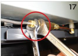
Using the other 'olive' and 'nut', re-connect the fluid pipe to the one-way valve using a size 10 & 12 spanner to tighten.
