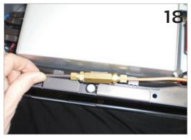
Now gently place the oneway valve assembly back behind the metal tabs of the chassis & underneath the Heat Exchanger
