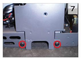
Now remove the 2 x M4x10 Black Taptite Screws holding the Vertical Strap in place at the top.
