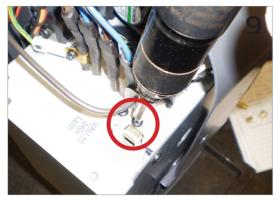
Now remove the 2 x M4x10 Taptites that hold the small metal bracket to the Heat Exchanger as shown.
