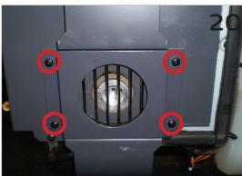
Re-attach the Trim Plate using the 4 x M4x10 Black Taptite Screws removed earlier.
