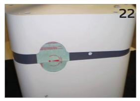
Slide L/H and R/H covers back into place ensuring tabs on inside of each cover are correctly aligned with the central vertical strap. Also, ensure that the earth leads are reconnected on both covers.
